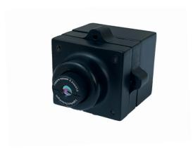
Utilizing the 80 x 80 LYNRED Micro80 microbolometer technology, the ATOM C80 is a low cost, compact, low power, shutter-less thermal imaging camera core suitable for a variety of applications. Two modular interfaces (USB and SPI) are available. Additionally, this camera core is equipped with on board NUC continuous algorithmic correction requiring no shutters or periodic correction.
