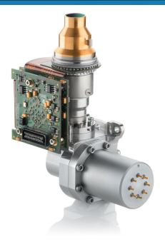
LEO-LP is a "Low Power" LEO thanks to an improved HgCdTe material enabling operating temperature +30K above the standard LEO product.
