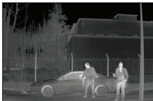
Figure 1: Thermal image obtained with 1024x768 a-Si microbolometer detector shows both high sensitivity and resolution. Courtesy ULIS.
